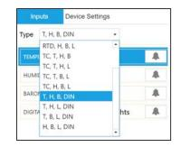
The SS-002-0 offers a configurable choice of one external thermocouple, RTD, or DIN (contact closure).
