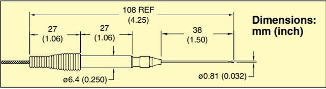
**Thermocouple Probe Model HYP2 and HYP5**
