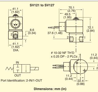
Wetted Parts: Stainless steel. copper and seal Medium: Liquid or gases Max Static Pressure: 1.5 times max psid, vacuum (>5 microns ABS) Ambient Temp: -9 to 50°C (15 to 122°F)
