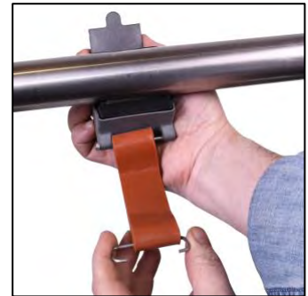
Figure 2: Mount the HANI™ Sensor
