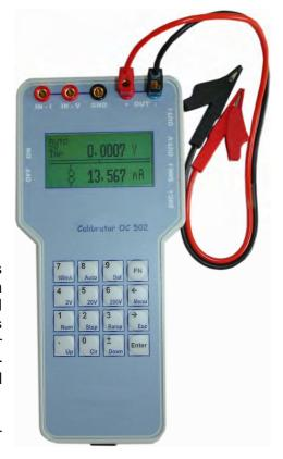
The instrument is supplied from internal battery and permits an uninterrupted operation of 3-4 hours with the output current between 0 and 20mA. For higher output currents up to 100mA the calibrator has to be connected to the charger. When the display shows BAT of the battery capacity, the calibrator has to be connected to the charger.
