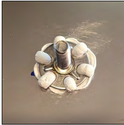
Figure 11: Evenly distribute the epoxy across the top of the stud base
