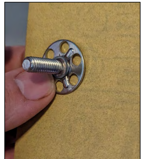
Figure 7: Sand the adhesive studs
