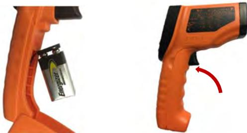
2. Attach a 9V battery (provided) to the black connector inside. The battery should snap into place. Swing the front of the handle back upwards to close the unit.
