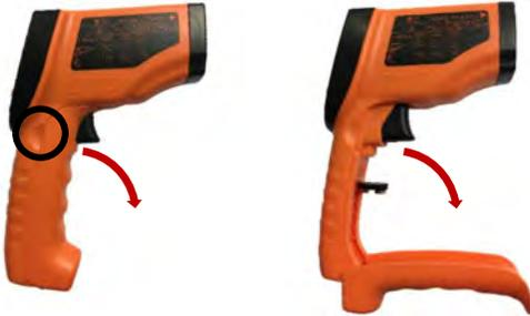
1. Locate the notches on the side of the unit's handle and pull the front of the handle forwards as shown above.
