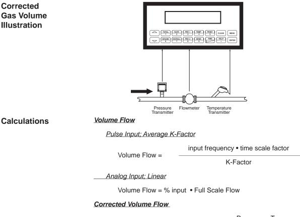
Corrected Volume Flow = Volume Flow •  $\frac{P}{P_{ref}}$  •  $\frac{T_{ref}}{T}$  •  $\frac{Z_{ref}}{Z}$
