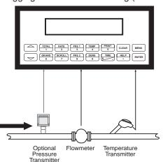
Monitoring corrected volume flow and total of any liquid. Flow alarms are provided via relays and datalogging is available via analog (4-20mA) and serial outputs.
