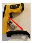
Insert the 9V battery into the battery holder.
