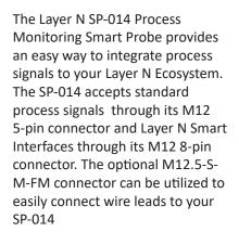
Each of the 3 process inputs may be independently configured as 0-24 mA or 0-1.0  $V_{\text{DC}}$  inputs.
