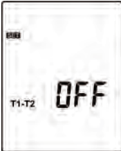
(5) Fig.5 Set T1-T2 subtraction mode.
