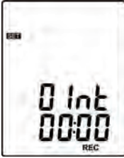
(2) Fig.2 Set interval time for data logging.
