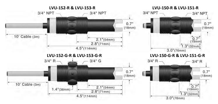
⚠ The sensor should be installed so that the liquid will drip out of the gap when the sensor becomes dry.
