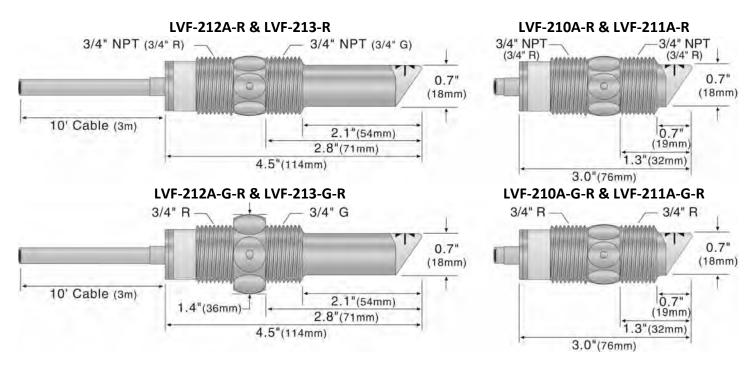
⚠ The Optic Leak Detector cannot detect the presence or absence of specular application liquids that reflect light (such as milk), or viscous liquids (such as paint) that form a coating on the sensor tip.
