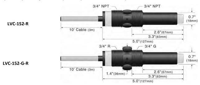
The sensor's operation may vary based on the dielectric properties of various application liquids. The LVC-152 series sensor is factory-calibrated to be used with liquids with a dielectric value between 20 and 80. Liquids with a dielectric constant less than 20 will not be detected by an LVC-152 series sensor.
