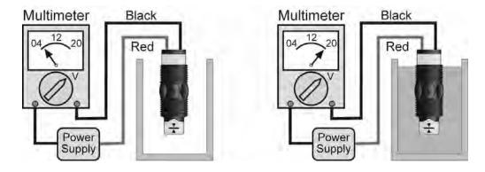
**Example:** Testing the LVU-150 series with a multimeter set to read resistance (ohms). When wired NO [Red to (+)], the meter will read O.L when dry and will read some small amount of resistance (ex. 0.2 Ohms) when wet.
